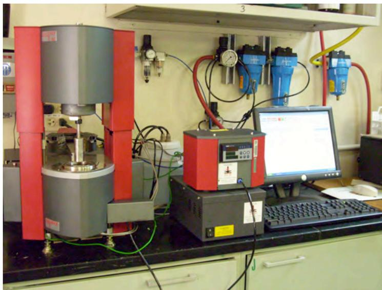
Figure 3.14 Rheometer equipment setup
