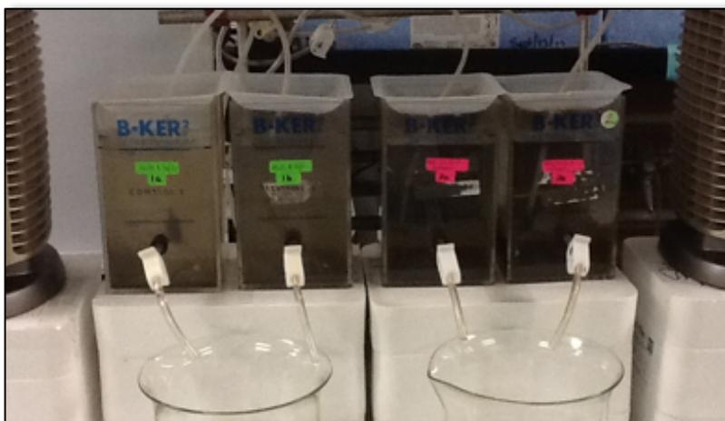
Figure 12: Lab-Scale SBR Experiment (Left to right: reactors 1a, 1b, 2a and 2b)
