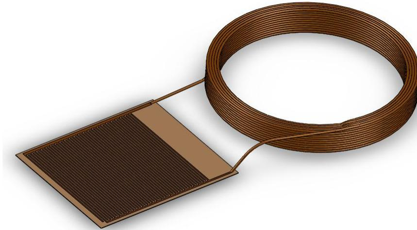
Figure 1–3: Schematic Interdigital Pressure sensor
