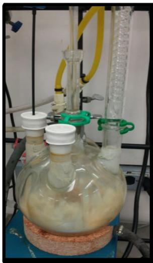
**Figure 8.11** Set up of the arylation reaction.
