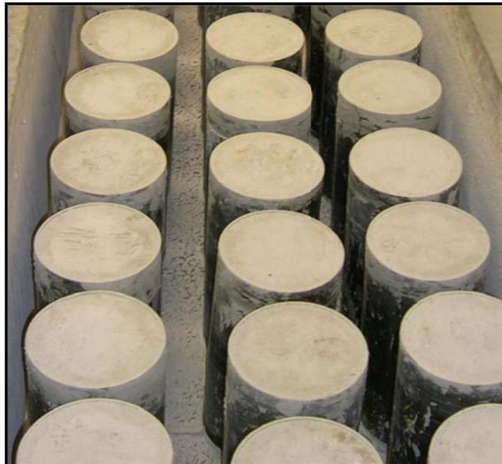
**Figure 3-12: Curing of CFFT under laboratory ambient conditions.**
