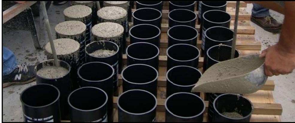
**Figure 3-2: Elaboration of control concrete cylinders.**
