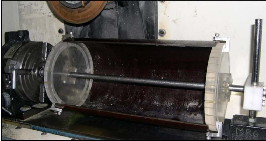
**Figure 3-8: Cut fixture for axial test samples.**
