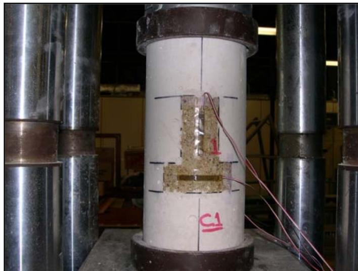
**Figure 3-4: Axial compression test of concrete cylinder.**
