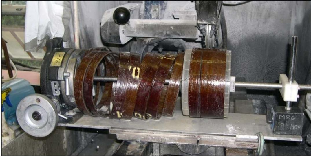
**Figure 3-6: Hoop tension test samples.**
