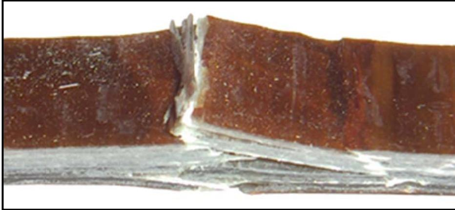
**Figure 4-24: Picture of baseline sample tested in axial compression.**
