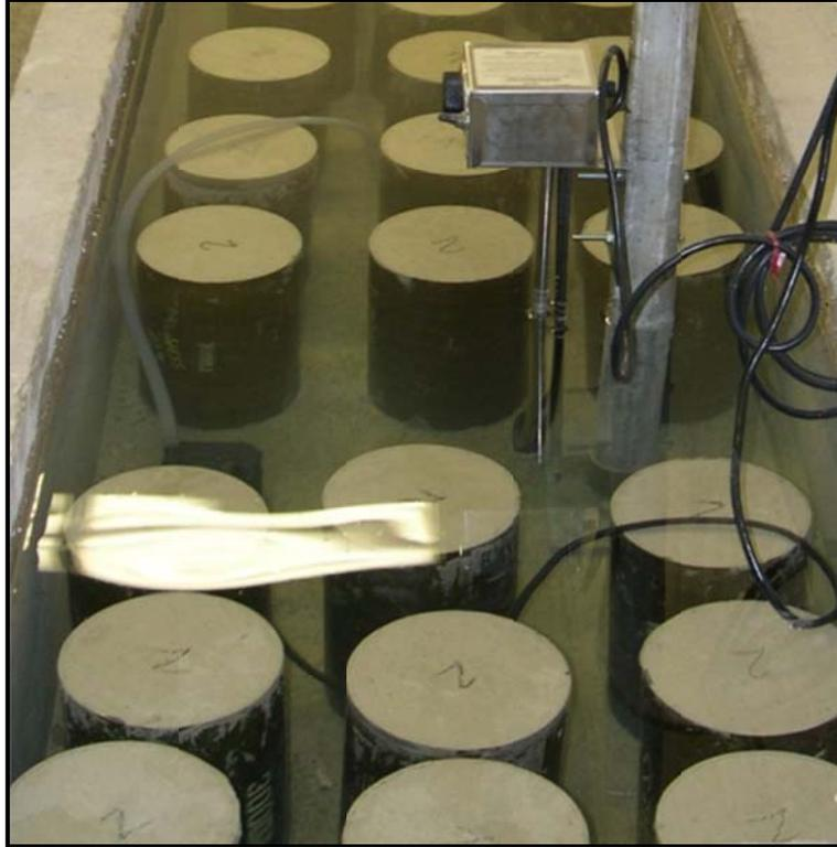
**Figure 3-13: Aging of CFFT in water at 30°C.**
