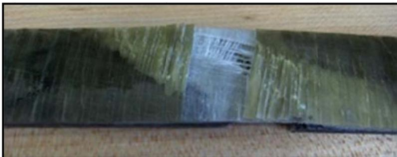
**Figure 4-20: Picture of baseline sample tested in axial tension.**
