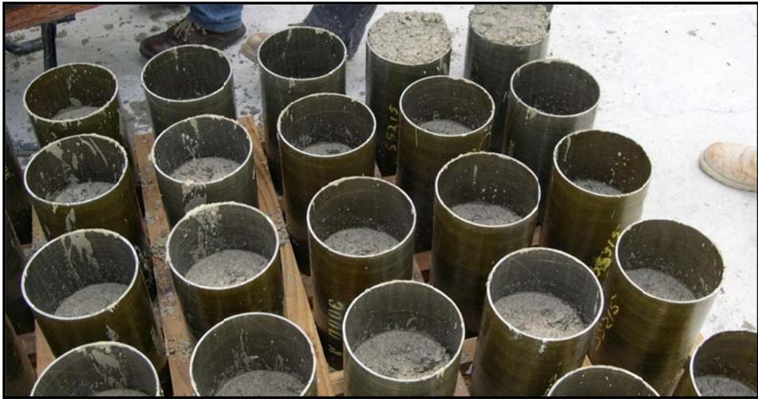
**Figure 3-11: Filling of FRP tubes with concrete.**
