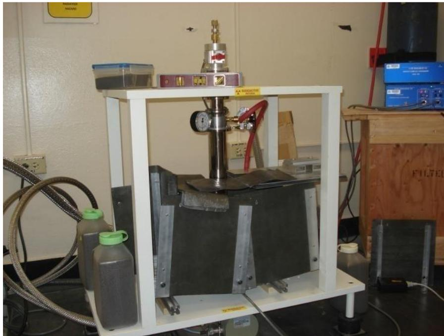
**Figure 31.** WEBRES spectrometer operating in the transmission mode, with  $^{57}\text{Co}$  source in a Rh matrix (Ritverc, GmbH).
