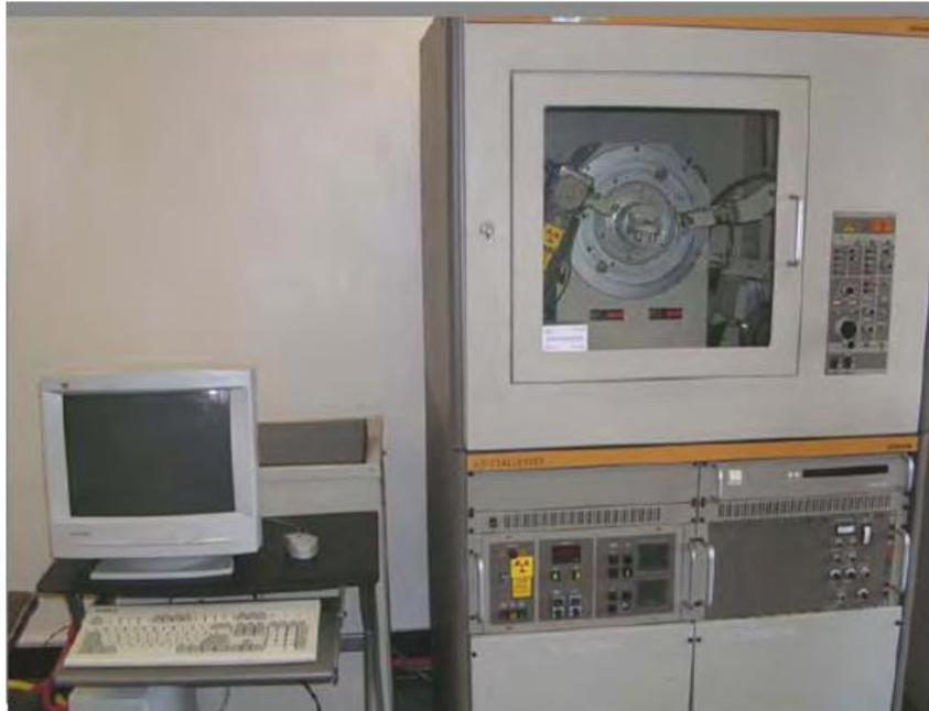
*Figure 24. Siemens D500 X-Ray Diffractometer.*
