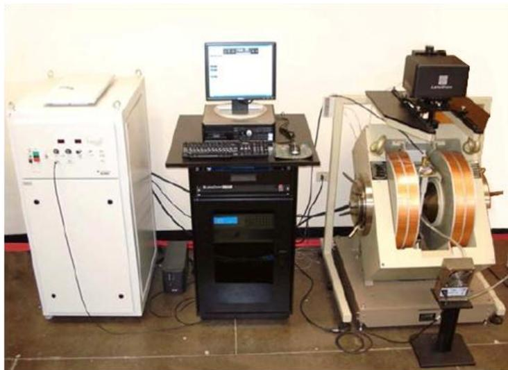
**Figure 27.** *Lakeshore 7400Series Vibrating Sample Magnetometer.*
