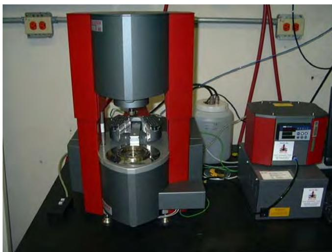
Figure 4.5. StressTech rheometer
