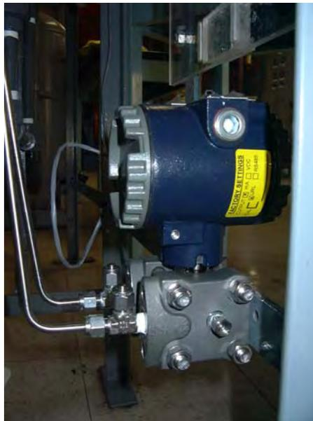
Figure 4.3. Differential pressure transducer
