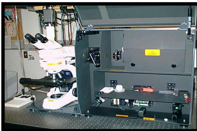
Figure 18. Renishaw Raman Microspectrometer (RM2000) with Leica objectives with 10x magnification used.
