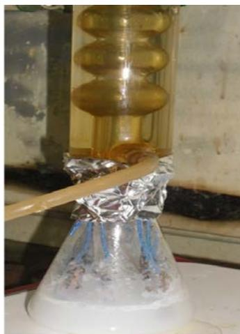
Figure 13. System used for ZnO NRs synthesis by wet chemistry method.
