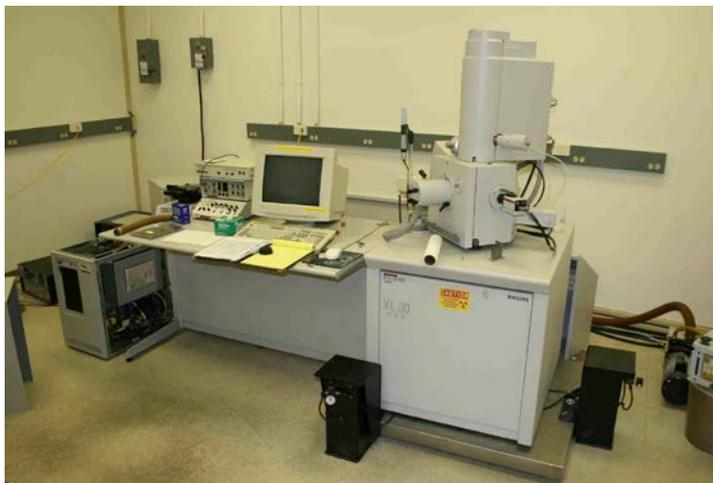
Figure 16. Image of a Philips/ FEI, XL30s, FEG SEM / Phoenix EDAX located at the Lab of Hewlett Packard-PR – Aguadilla.
