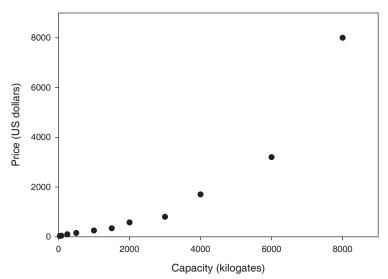
Figure 2–3: Price vs. capacity for Xilinx Virtex 2 FPGAs. Source: www.digikey.com
