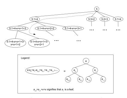
Figure 5–3: Part of a breakdown strategy mega-tree for 32-point FFT.
