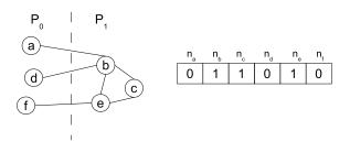
Figure 4–8: Example of a chromosome encoding for a bipartitioning solution.
