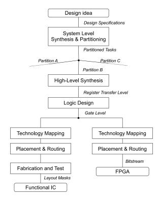
Figure 2–1: Flow for Computer Aided Design for VLSI.
