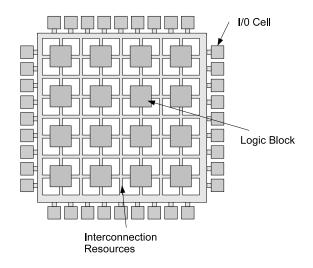
Figure 4–14: FPGA components.
