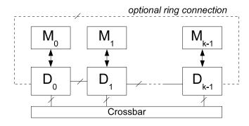
Figure 2–2: General architectural model for a distributed hardware architecture.
