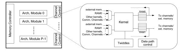
Figure 4–12: Device-level architectural model and block diagram for an FFT module.
