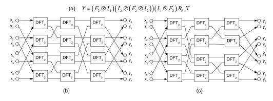
Figure 4–2: KPA formulation and two isomorphic dataflow graphs.
