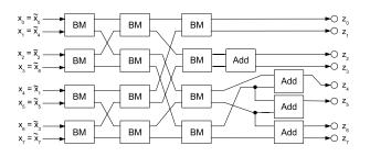
Figure 5–9: 8-point HT-DCT using a single functional primitive that performs both the BM and post-processing functionalities.
