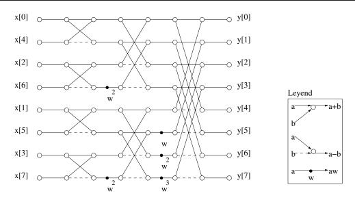
Figure 2–5: Data flow for an 8-point FFT. Dashed lines represent operands that will be subtracted. Filled dots represent multiplication by twiddle factors.
