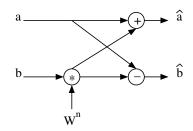
Figure 2–4: Dataflow graph representation of the radix-2 butterfly.
