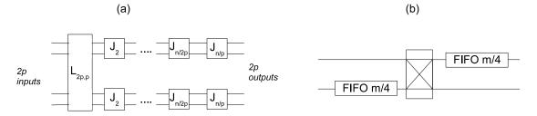
Figure 2–10: (a)A vertically-folded  $L_{n,n/2}$  permutation with 2p ports. (b) Detail of the  $J_m$  component, proposed by Takala, et al.[58][59].
