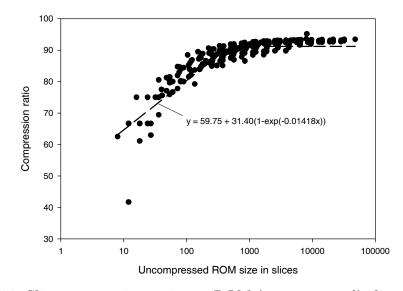
Figure 4–16: Slice compression ratio vs. ROM (uncompressed) slice utilization.
