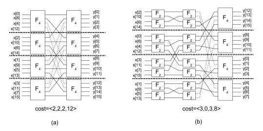
Figure 4–11: Two formulations for an 16-point FFT, representing different granularities. Horizontal dashed lines represent the partition boundaries.
