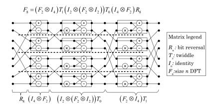
Figure 4–10: 8-point DFT Cooley-Tukey formulation, showing initial linear horizontal partition.
