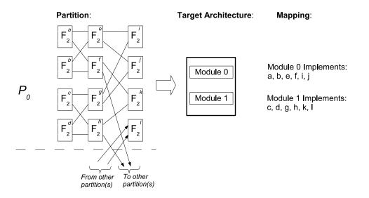
Figure 4–13: Example mapping of a DFG partition to a device with two architectural modules.
