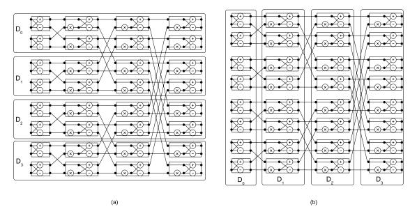
Figure 2–6: A one-to-one mapping of a 16-point FFT to a 4-FPGA platform.
