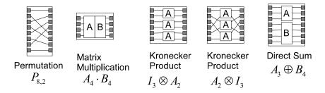
Figure 4–4: Common KPA operations and their KA-component representation.
