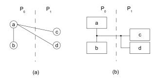
Figure 4–6: (a)Graph and (b)hypergraph representations of a circuit netlist.
