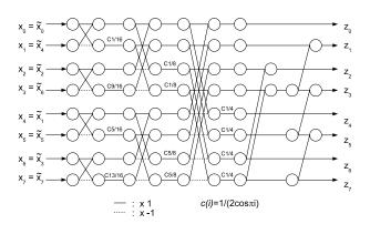
Figure 5–8: 8-point HT-DCT [81] data flow graph.
