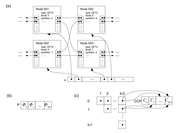
Figure A–11: Main DGP data structures.
