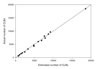
Figure 4–19: Actual vs. estimated slice utilization for various FFT sizes.
