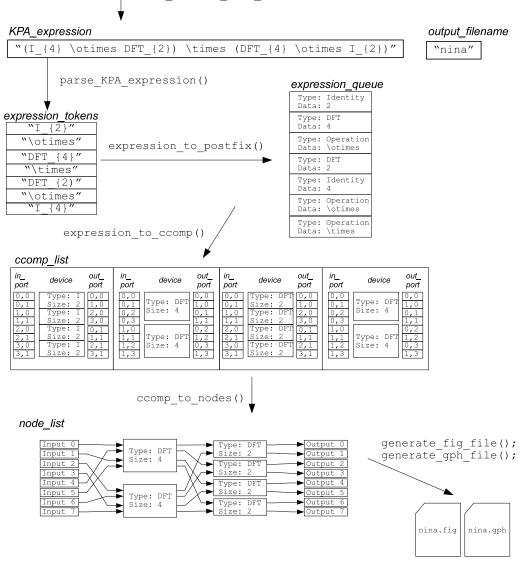
Figure A-4: Illustration of the effect of KTG functions.
