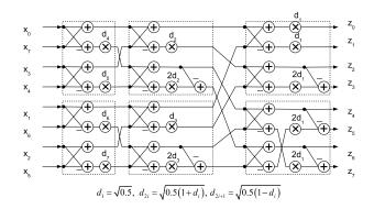
Figure 5–12: DFG for an 8-point NPS-DCT [1].
