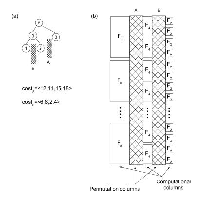
Figure 5–5: A split tree for a  $n = 2^6$ -point DFT and part of its corresponding DFG.
