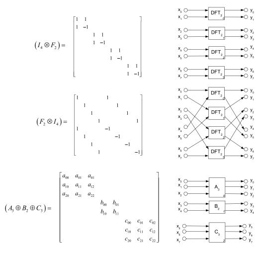
Figure 4–1: Several KPA sparse matrices and their corresponding data order topology DFGs.
