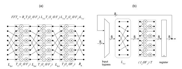
Figure 2–9: (a)An 8-point Pease FFT formulation and dataflow graph. (b) full horizontal folding [58]
