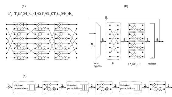
Figure 2–7: Folding of an 8-point FFT: (a) fully expanded DFG, (b) strict horizontal folding and (b) strict vertical folding.
