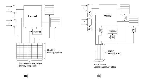
Figure 4–18: Two approaches for implementing module-level control logic (a)integrated, (b)distributed.
