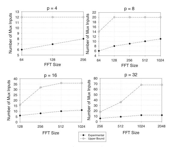
Figure 4–17: Experimental results for mapping of several FFT sizes to architectures with 4, 8, 16, and 32 modules.
