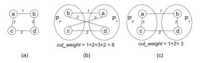
Figure 4–5: (a) Graph (b) a partition solution, (c) partition solution after swapping nodes a and b.
