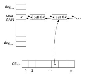
Figure 4–7: Bucket structure used in the Fiduccia-Mattheyses algorithm [68]
