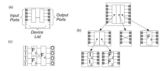
Figure 4–3: (a)The KA-component data structure, (b) KA-component representation and (c) derived DFG for sample formulation  $F_4P_{4,2}(I_2 \otimes F_2)$
