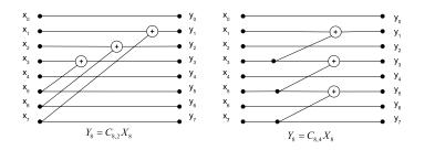
Figure 5–6: Dataflow graphs of  $C_{8,2}$  and  $C_{8,4}$  matrices.
