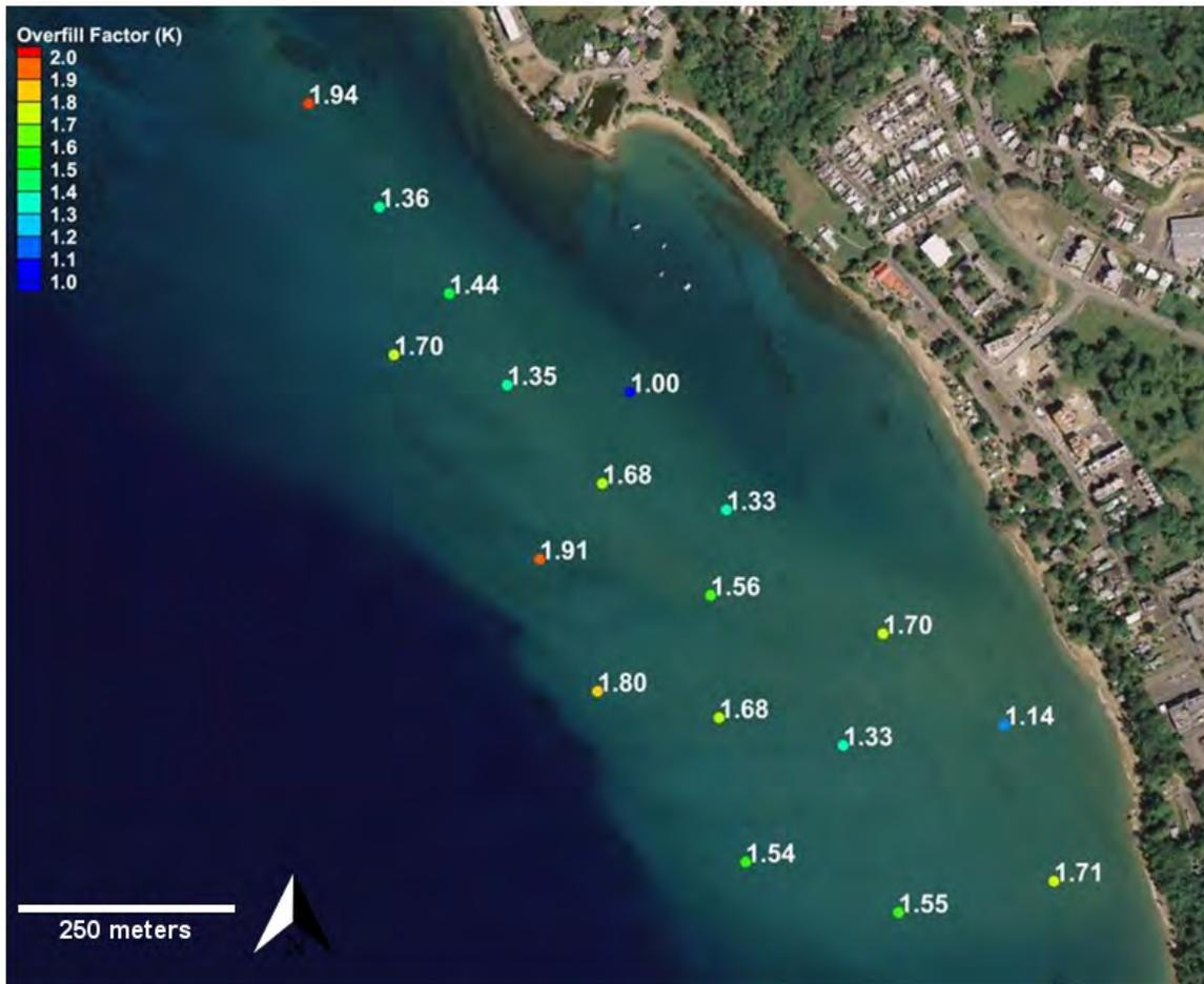
**Figure 3.23:** Dean's overfill factor for the mean grain size of Bajo Blanco and the mean grain size from eroded beaches in Rincón.
