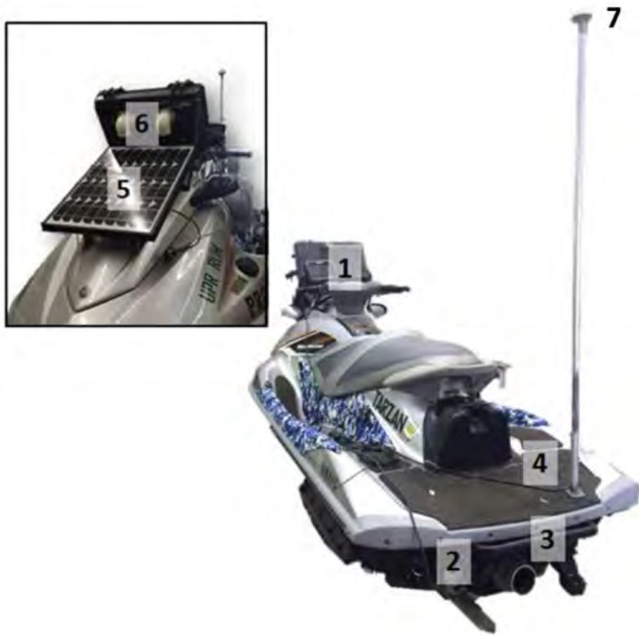
**Figure 3.1:** Personal watercraft instrumentation: (1) Lowrance HDS-7 Gen2 Touchscreen; (2) StructureScan HD Sidescan; (3) Sonarmite BT echosounder system; (4) GPS support pole; (5) solar panel; (6) watertight laptop case; (7) YUAN10 GPS receiver (modified from Chardón, 2013).
