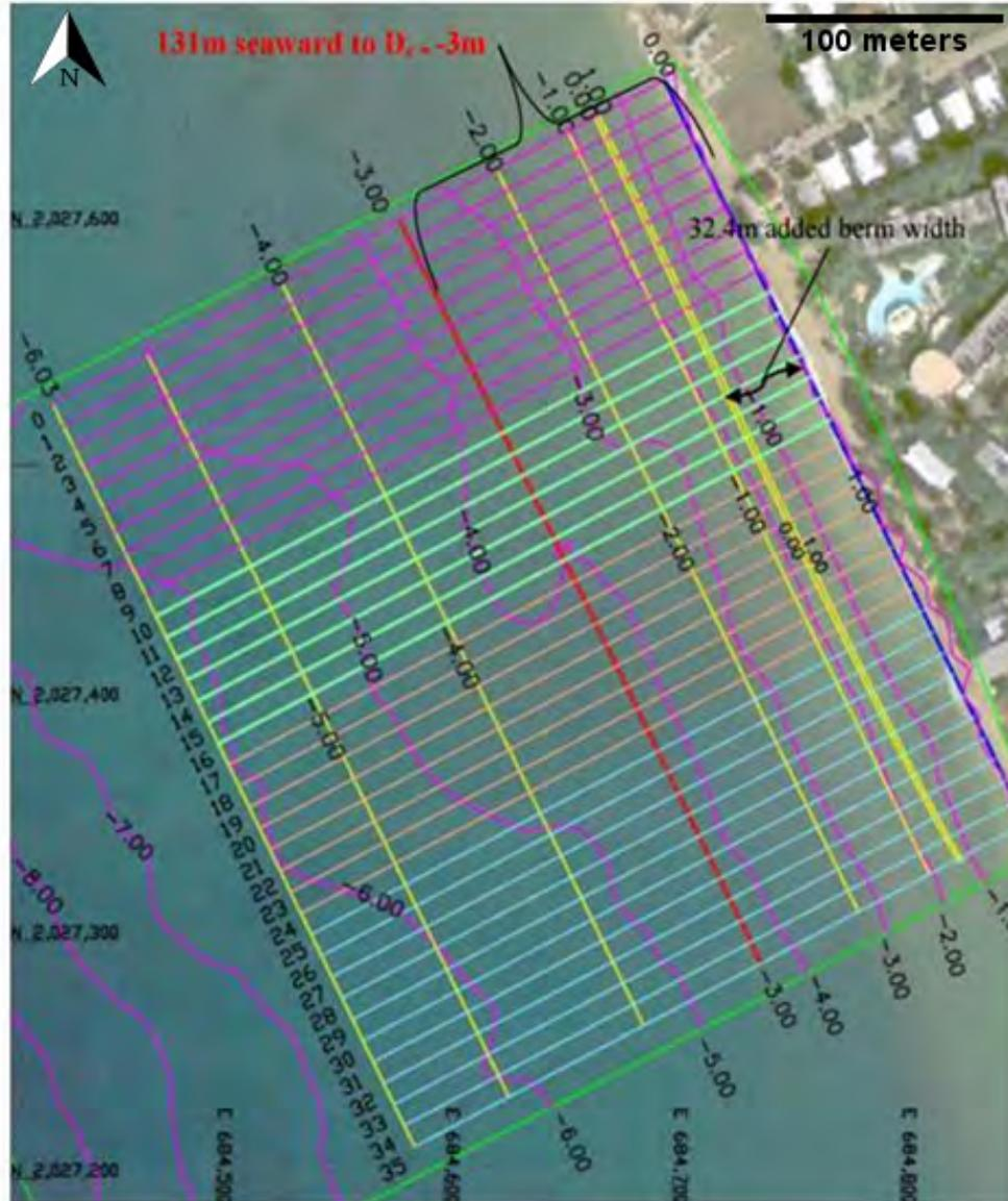
**Figure 3.21:** Schematic showing existing bathymetry contours (magenta) along with the depth of closure (red) and the calculated beach profiles elevation (yellow) (from Salas, 2014).
