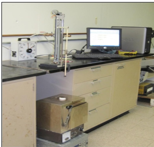
Fig. 4.6 Experimental Setup for Rapid Thermal Annealed used in this work. (Dr. M. S. Tomar's Laboratory, UPR-M)
