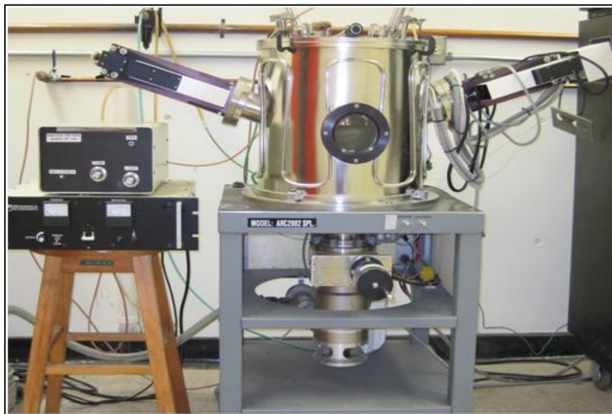
Fig. 4.5 Sputtering system setup used of this work. (Dr. M. S. Tomar's Laboratory, UPR-M)
