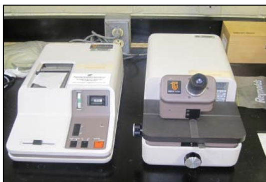
Fig. 6.6 Tencor-100 Profilometer Equipment used for this experiment (Dr. F. Fernández's Lab., UPR-M)
