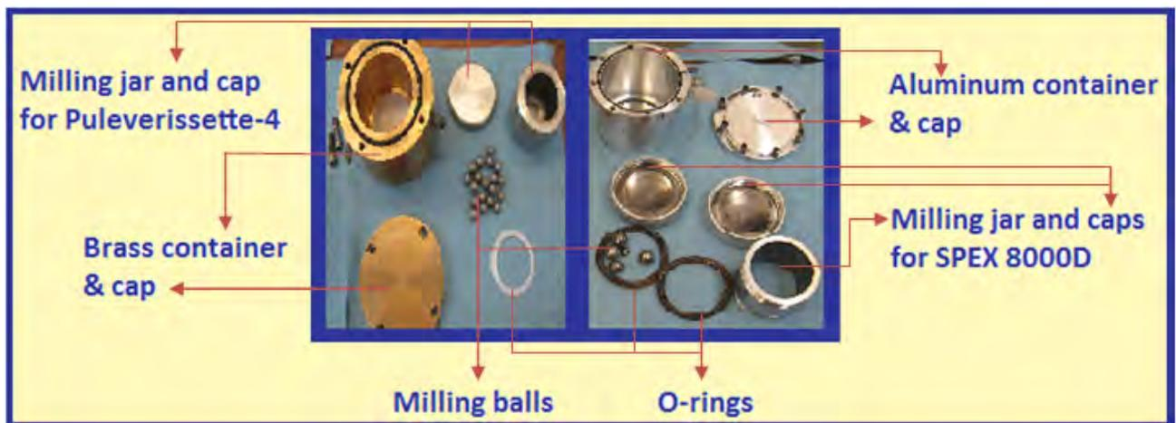
Figure 3.8 WC-Milling jars, control atmosphere container, milling balls and O-rings used in this work.
