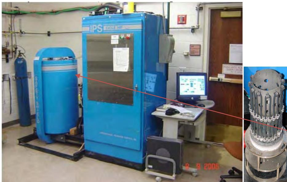
**Figure 3.11** Hot Isostatic Press use in this work ,from D. Rodrigues Jr [26].
