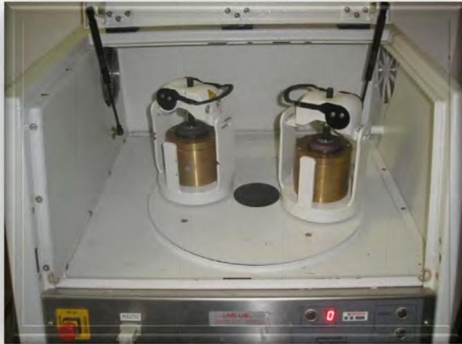
**Figure 3.4 Fritsch Pulverisette-4 with the two special made brass can.**
