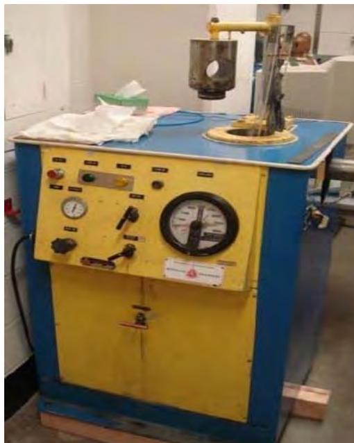
**Figure 3.10** Cold Isostatic Press use in this research work ,from D. Rodrigues Jr. [26]
