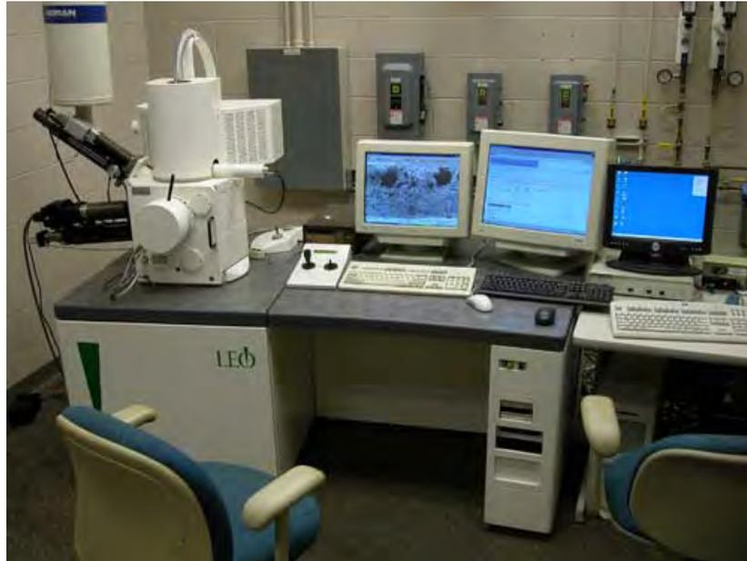
**Figure 3.19** A fully digital LEO GEMINI 1530 SEM with field emission electron gun, full orientation imaging based on backscattered electron Kikuchi patterns, and full EDS and control . University of Wisconsin-Madison, Material Science and Engineering Building MS&E – 171.
