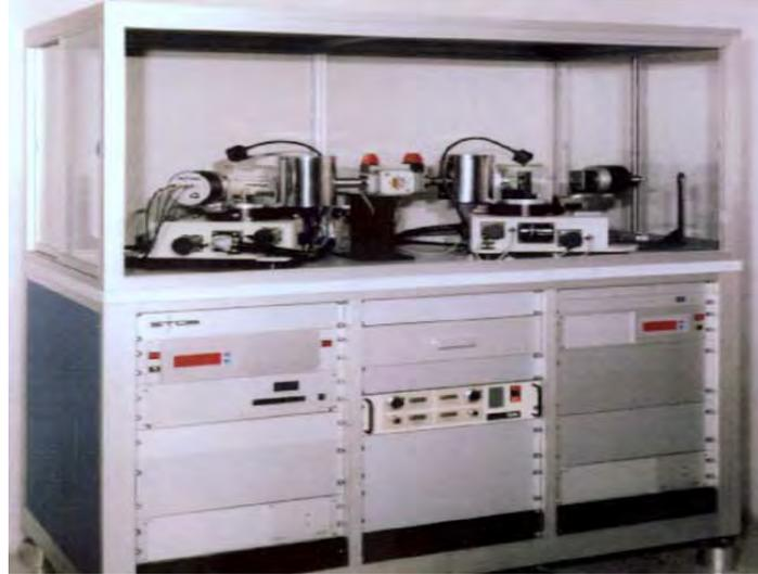
**Figure 3.18** STOE X-ray diffractometer. University of Wisconsin-Madison, ERB - 1128
