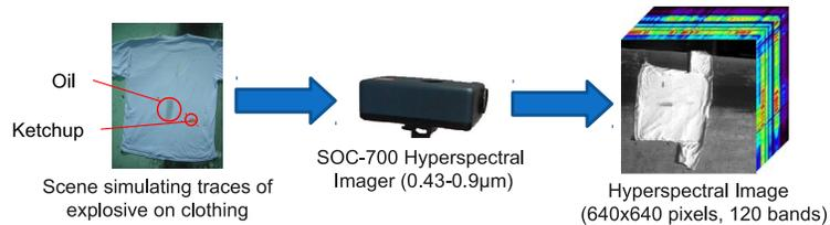
Figure 4–1: Phantom image generation for the experiments: a hyperspectral image was collected using a SOC-700 imager.
