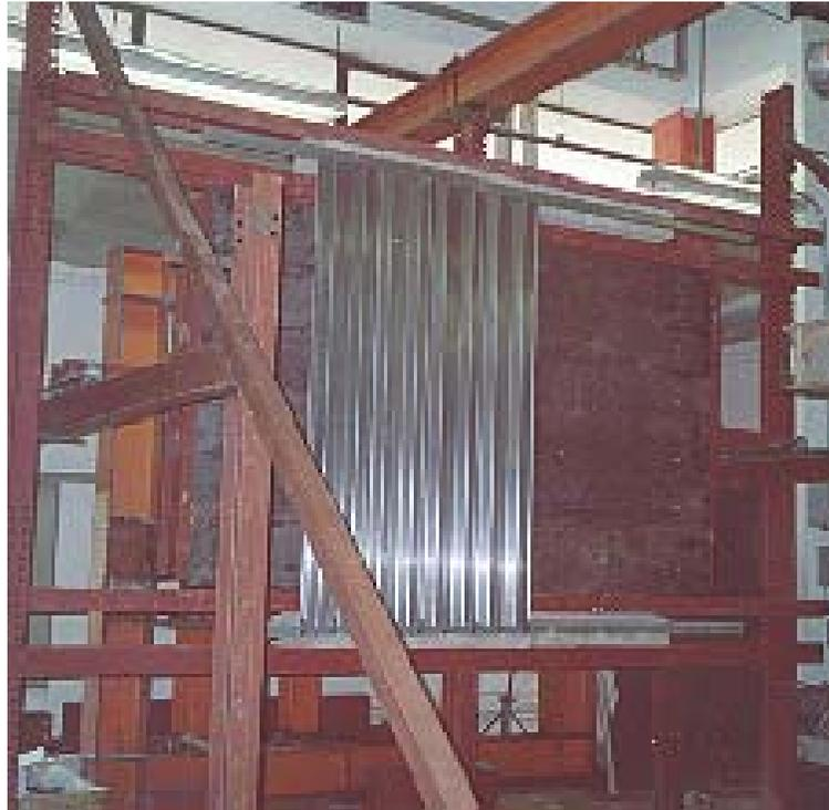
**Figure 2-5.** Final Assembly: Rigid frame with four shutter panels attached
