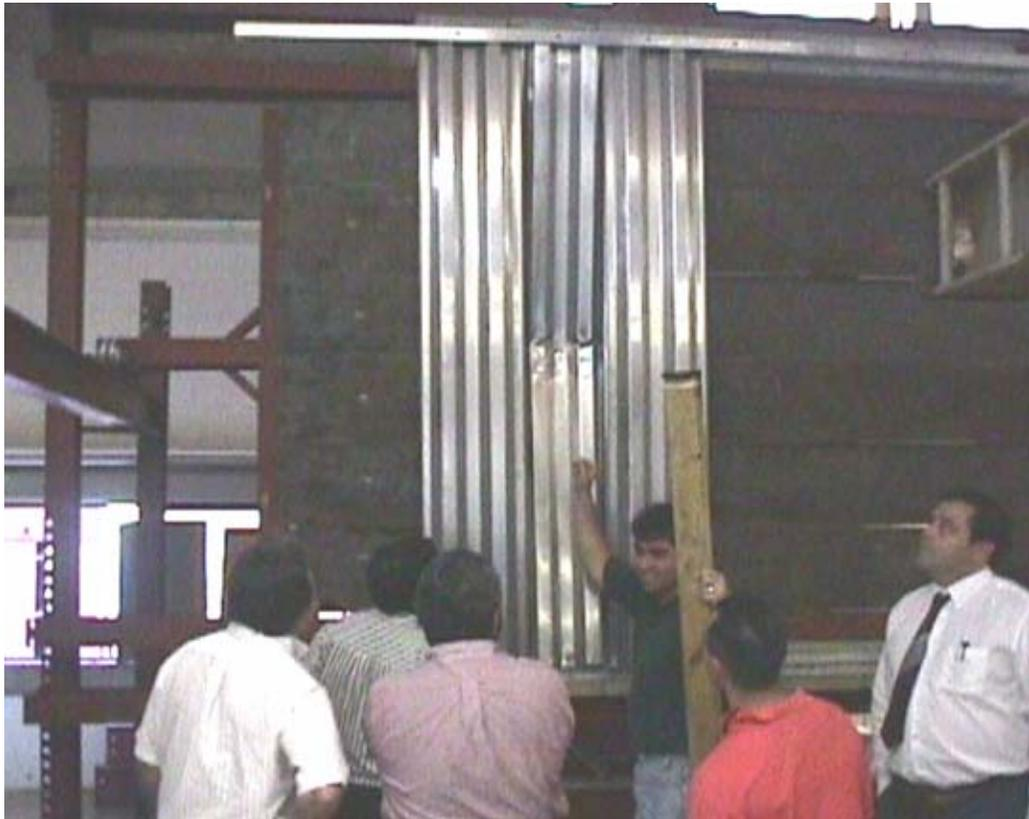
**Figure 3-15.** Permanent deformation at middle span
