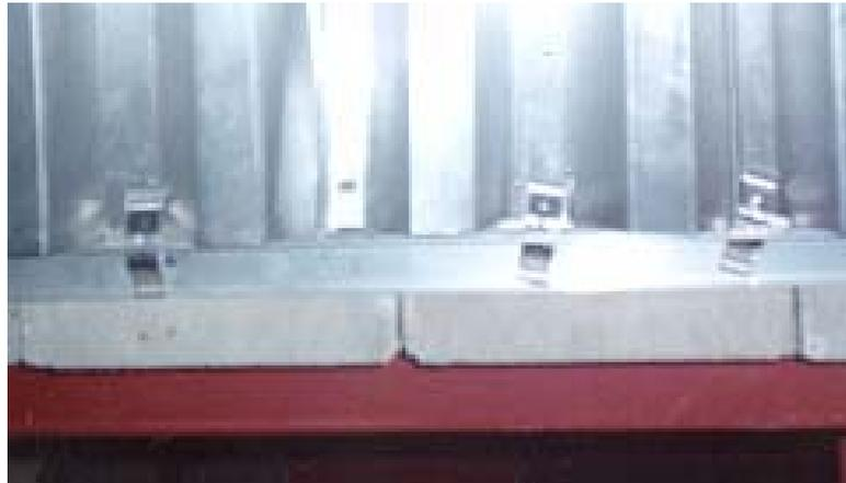
**Figure 3-12.** Rotation and lost of clips due to impact
