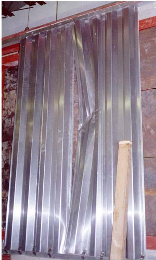
**Figure 3-11.** Permanent deformation at middle span
