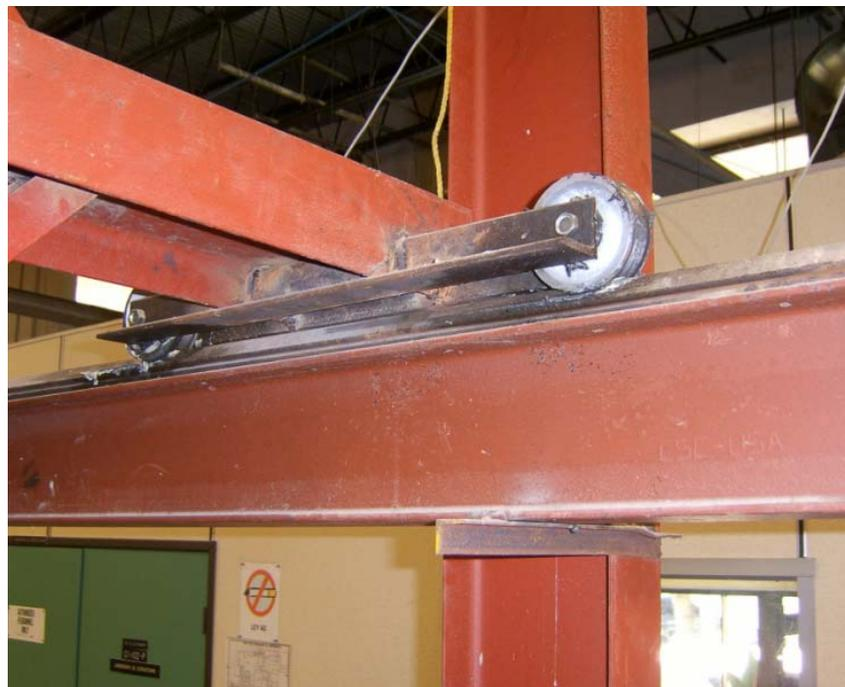
**Figure 2-9.** Steel Wheels Connection
