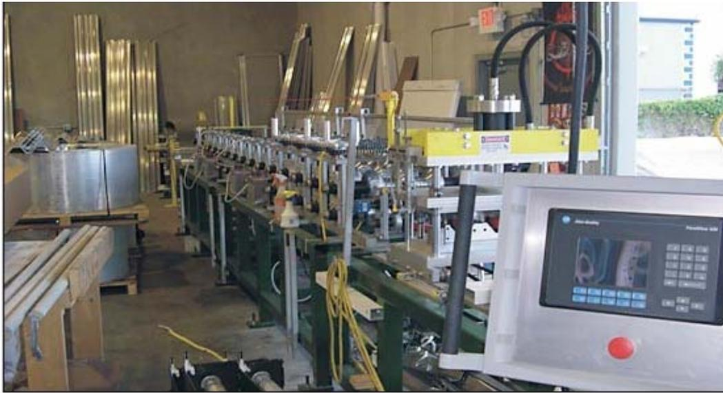
**Figure 6-19.** Equipment used in the storm shutter panel's fabrication (JA, 2008)
