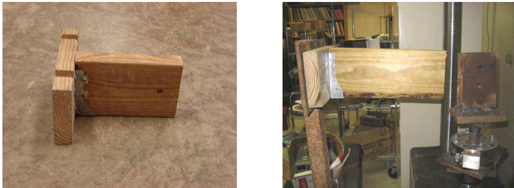
Figure 7.1 – Dynamic load test set up for roof-to-wall connections
