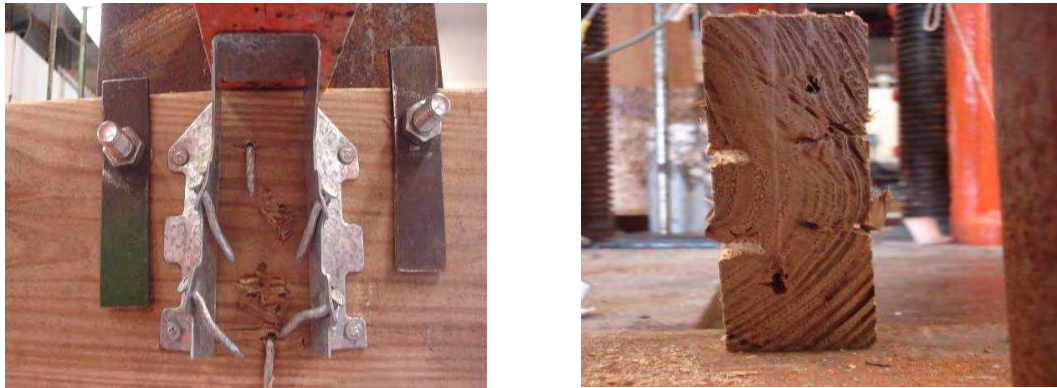
Figure 7.4 – Damages in full-scale test
