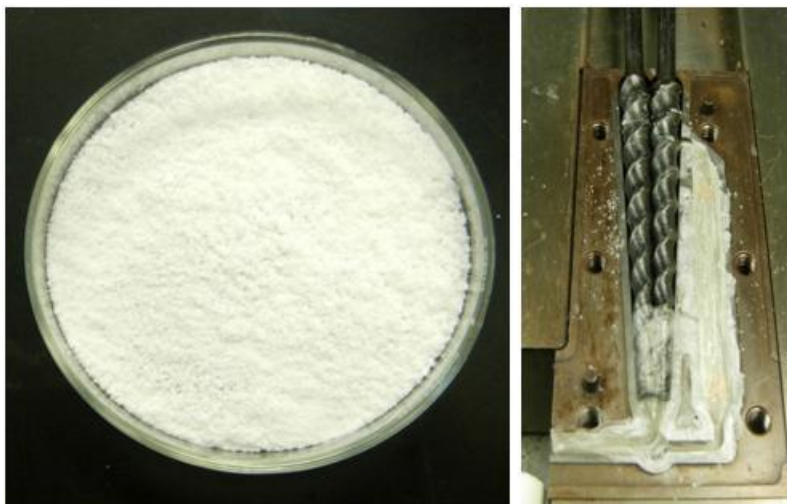
Figure 4:1: The image in the left is a blended mixture of HPC with plasticizer, the image to the right is the mixture at the extruder.
