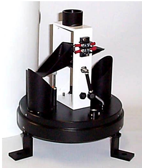
Figure 2.1 Inside view of a state of the art tipping bucket rain gauge (Source: http://www.novalynx.com/images/tipping-bucket-large.jpg ).
