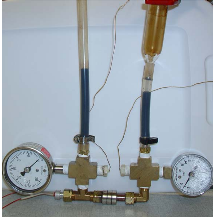
Figure 5.5 Magnetocaloric pump prototype during a test.
