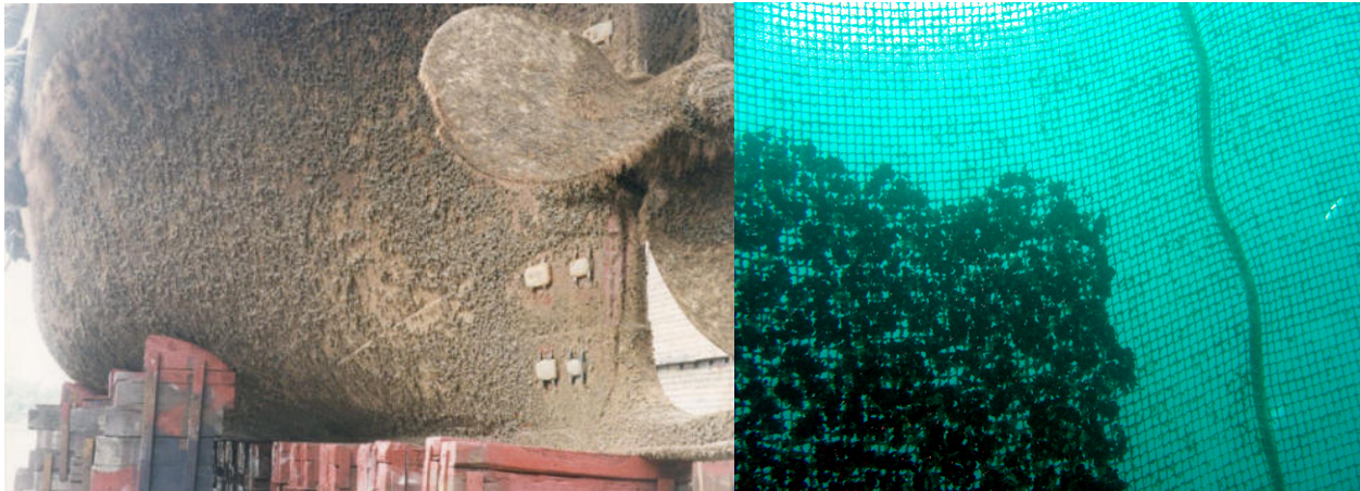
Figure 1. Biofouling growing on a ship's hull and aquaculture net cage. (From AMBIO 2006, and FAO 2007a, respectively.)
