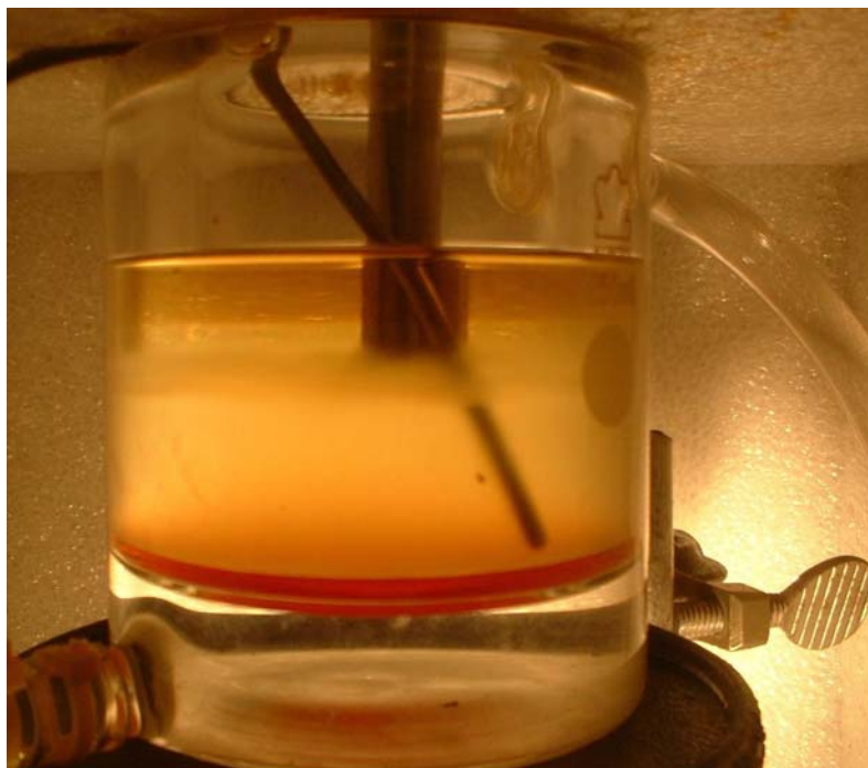
Figure 24. End of reaction, reactants and products without ultrasonic agitation
