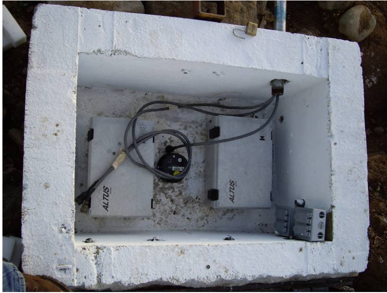
Figure 3-9. Triaxial Sensor and MAKALU Digital Recorders on the Crest
