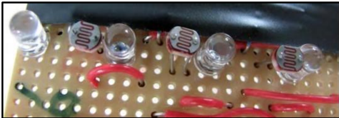
Figure 9: The Sensor Bar of the Line-following Robot.
