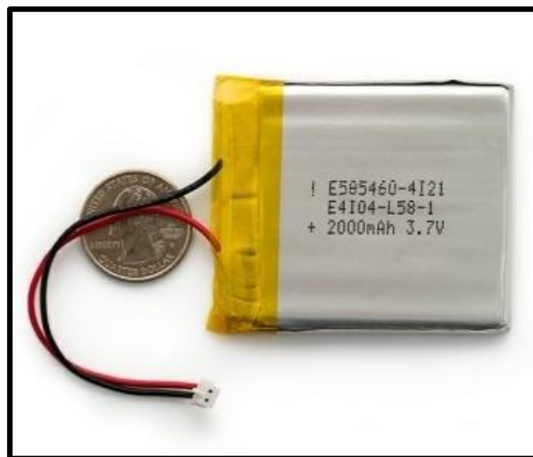
Figure 27: Rechargeable Lithium Polymer Battery. Image Provided by Sparkfun Electronics.
