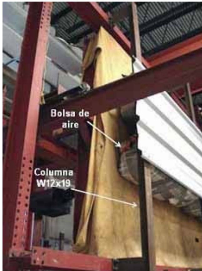
Figure 1 Wind pressure simulation by means of air bags in the experiments by
