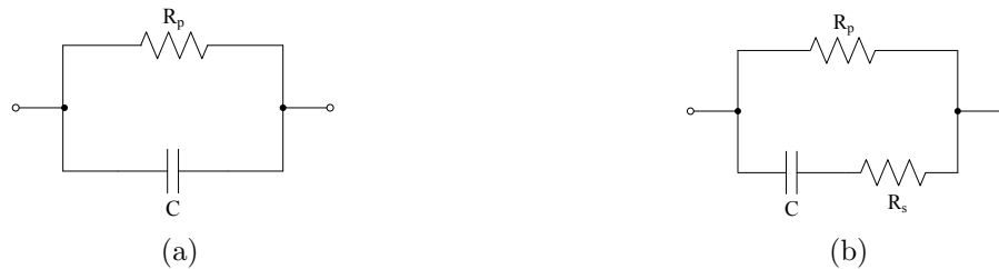
Figure 3-3: Low Frequency simple models for Capacitors : (a) Single resistance; (b) Shunt and series resistance
