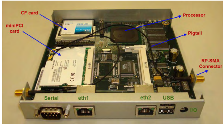
Figure 4.2: Hardware components of the Alix 2D2 board.
