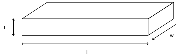
Figure 5–6: Geometrical parameters of a trace segment
