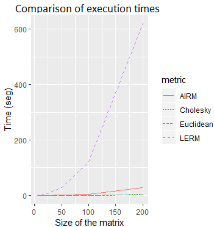
Figure 14 Comparative of execution times for the distance metrics varying the size of the matrix
