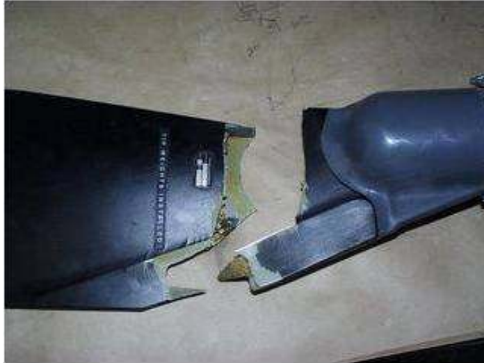
Figure 1.3: R22 Main Rotor fatal Blade rupture [4].
