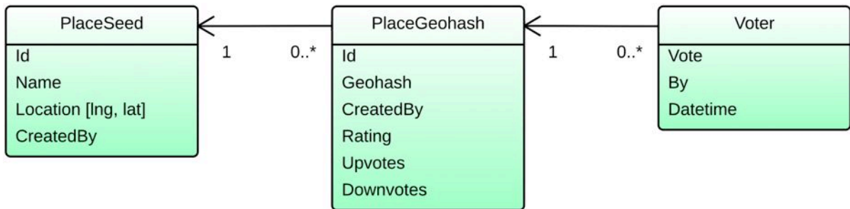
Figure 3.33 Relation between a Voter entity and the “evolved” PlaceGeohash entity (which relates to a PlaceSeed)
