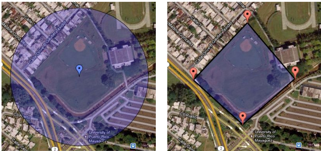
Figure 1.5 Geo-fencing alternatives done for a baseball park
