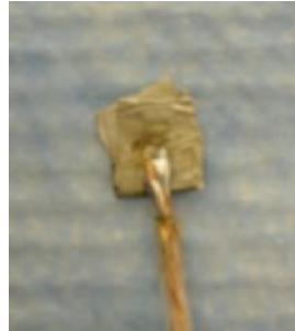
Figure 6: Electrode connection. A piece of Pt sheet was welded to insulated Cu wire.
