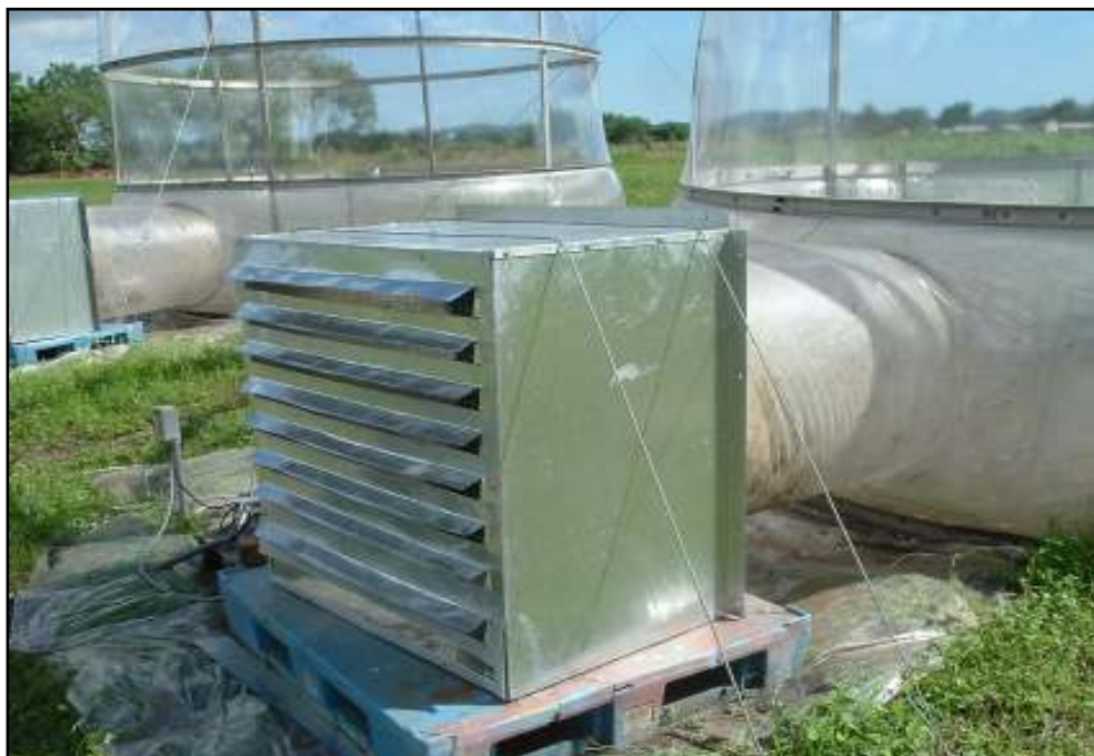
Figure A1. Chamber fan
