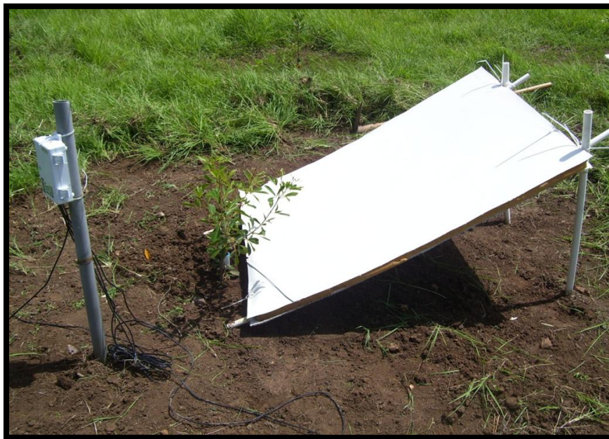
Figure 2. Dew condenser for providing water to a young Tabebuia heterophylla seedling, Cabo Rojo, Puerto Rico.
