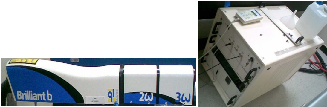
Figure F-4 UPRM Lidar laser unit (laser unit-left and power supply and cooling unit-right).
