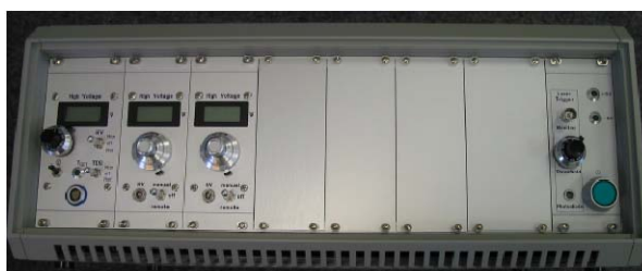
Figure F-9 Licel power supply unit.
