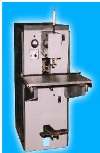
Figure 7.9 RF Welding System [41]
