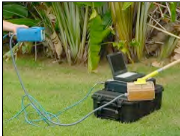
Figure 2.3 GSSI inc. SIR 20 GPR System
