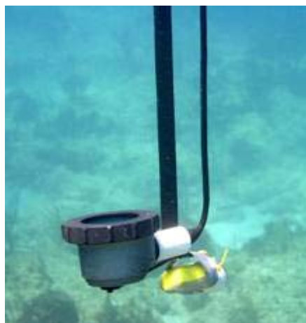
Figure 4b. Solar Light PAR quantum sensor PMA 2132 inside its underwater metal frame.
