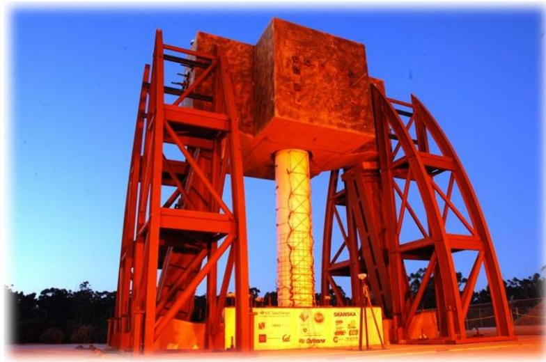
Figure 1.4. 3. UCSD column pre-test setup (UCSD report)
