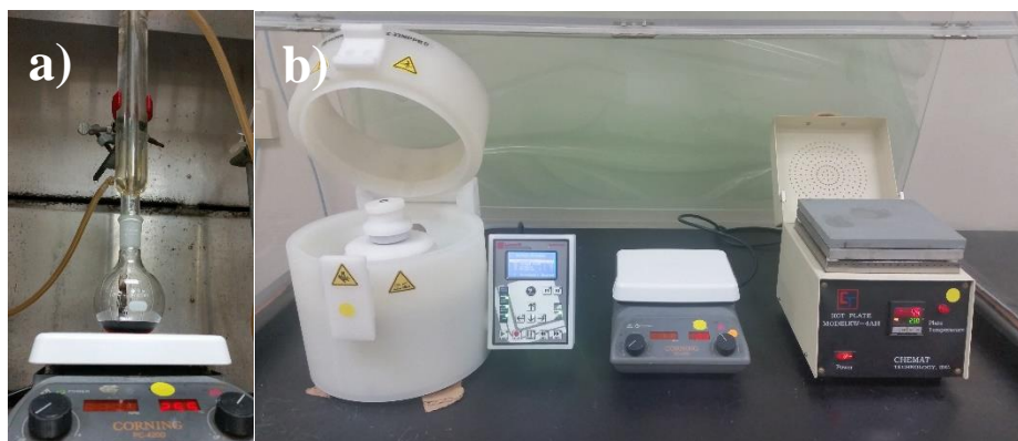
Figure 4.3 Setup for spin coating method employed for the synthesis of \text{Bi}_{(1-x)}\text{Co}_x\text{FeO}_3 thin films. a) Synthesis of initial solution. b) Spin coater and hot plates for coating/drying process of films.
