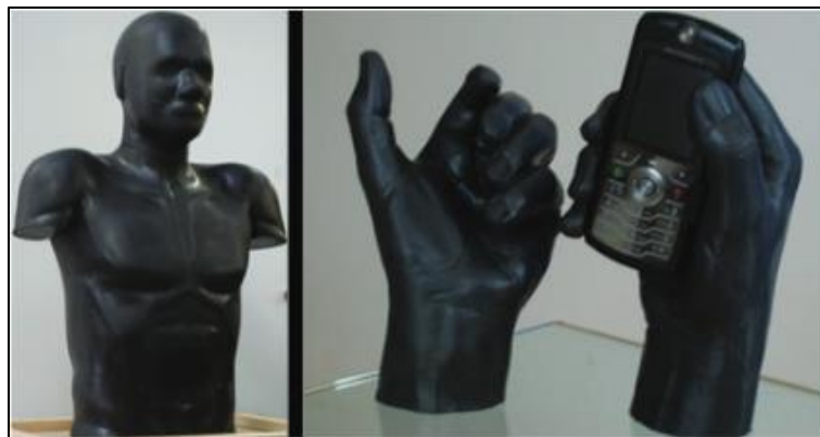
Figure 2.5 Solid Phantom of Carbon-loaded silicon rubber [1]
