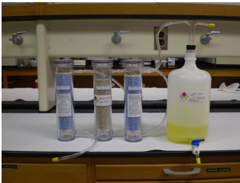
Figure 8. SMP buffer storage using drierite (blue) and ascarite cylinders to protect against CO 2 and H 2 O vapor contamination.
