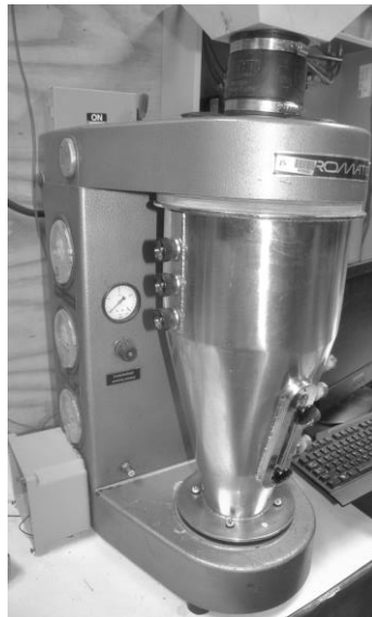
Figure 5. Batch fluid bed dryer (FBD) Aeromatic STREA-1™.
