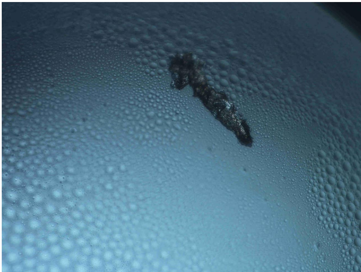
Figure 34. Microcrystal of HsKrr1 . The precipitant solution used was 50% PEG 3350 in 1.5 M triammonium citrate, pH 8. The crystal is growing at the interface of phase separation.
