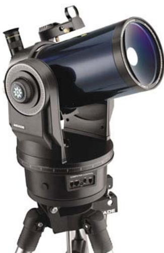
Figure 6. Reflective telescope employed to collect the Raman scattered signal.
