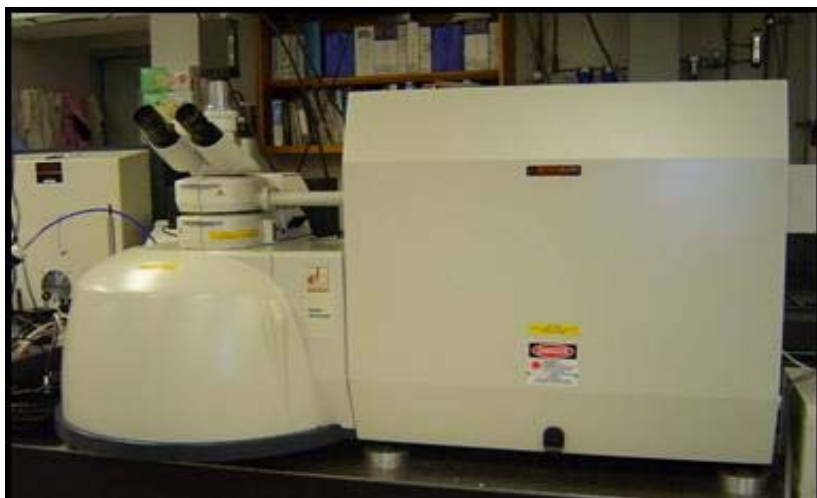
Figure 10. Renishaw Raman Microspectrometer (RM2000) with Leica objectives with 10x magnification was used.
