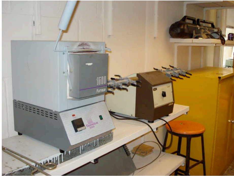
Figure 3.4: Equipment to heat the samples at temperature of 125° Cand175°C available at the University of Kansas.
