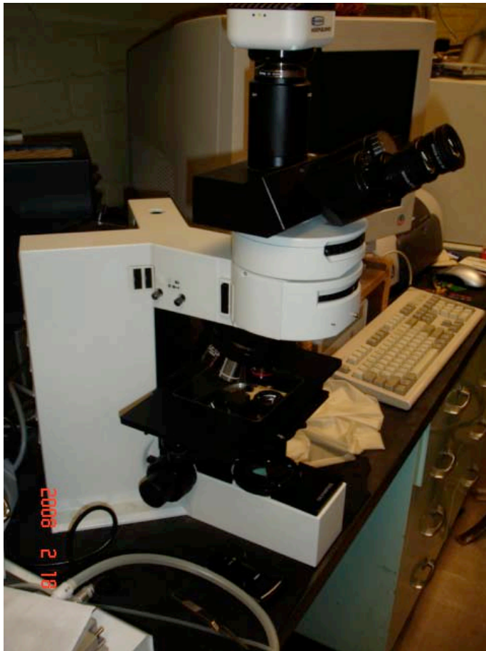
Figure 3.1: Petrographic microscope designed to observe fluid inclusions (University of Kansas).
