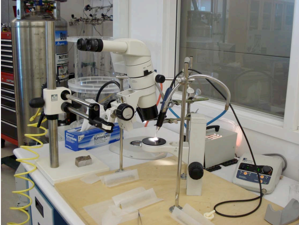
Figure 3.7: Microscope used to drill hand sample to obtain the samples of dolomites. Available at the University of Kansas.
