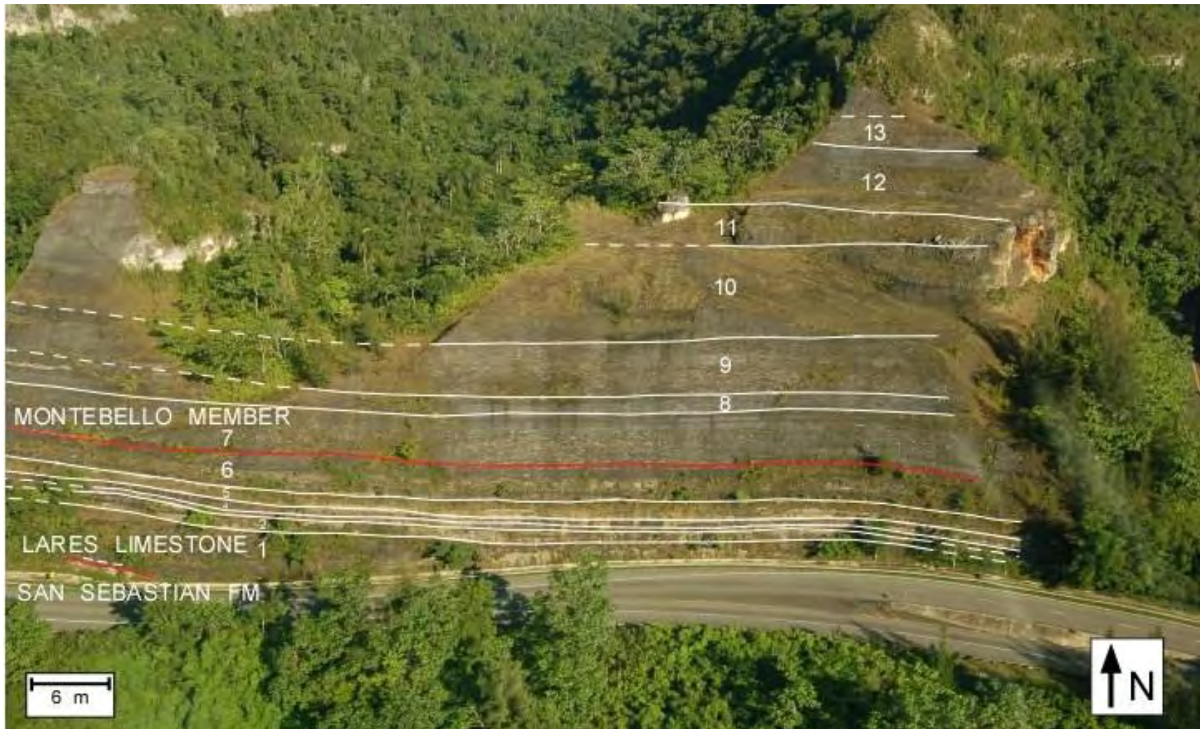
Figure 5.2: Photomosaic interpretation on PR-10 road outcrop. The red lines mark the lithologic contacts between units.
