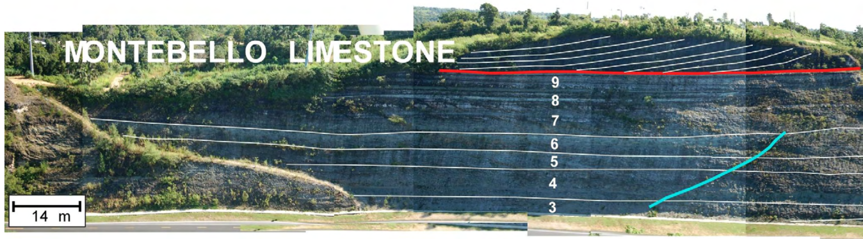
Figure 5.1: Photomosaic interpretation of PR-111 road outcrop. A. Complete PR-111 outcrop section and B. West-side PR-111 outcrop. The red lines mark the lithologic contact between units.
