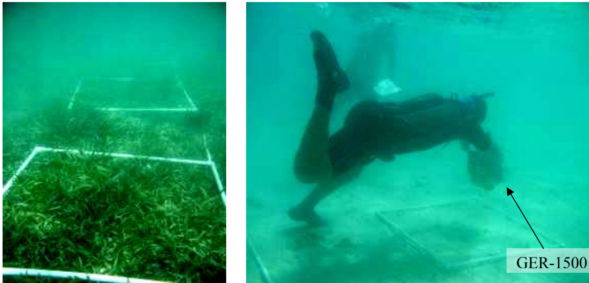
Figure 3.3 Underwater quadrant station for sea grass (left) and bottom albedo measurements with the GER-1500 Spectroradiometer in a waterproof housing (right). [6]
