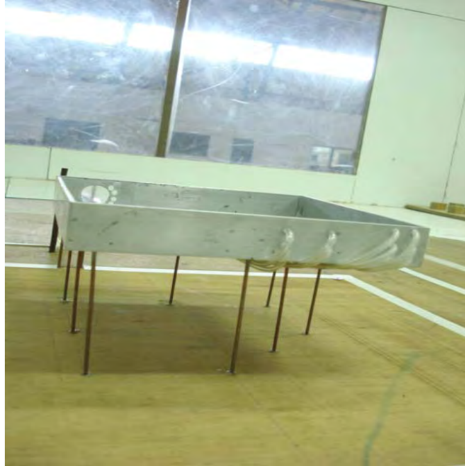
Figure 4.6: Model with parapets with PVC tubes and columns. (Photograph by the Author)
