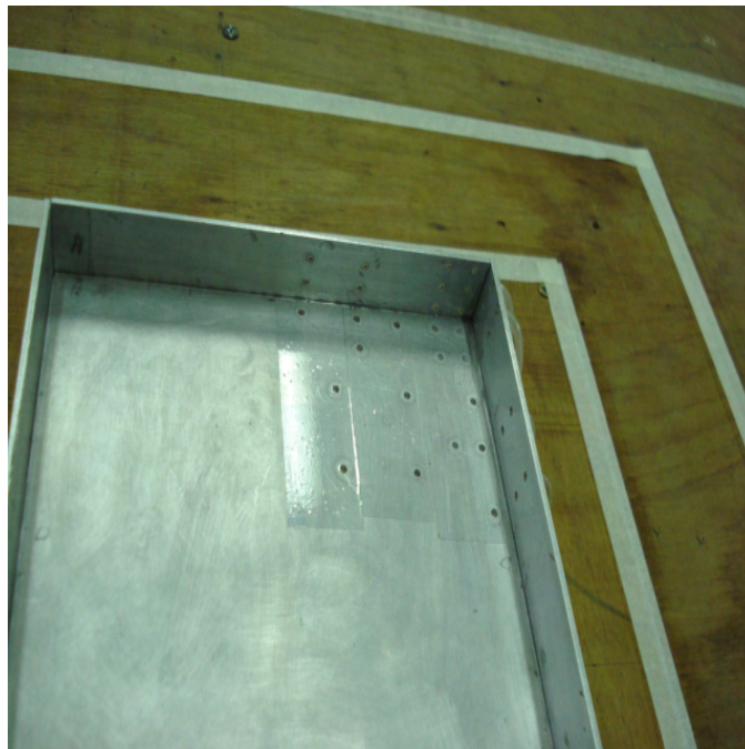
Figure 4.7: Top view of the model, showing the distribution of 16 pressure taps on the top surface of the canopy and parapets. (Photograph by the Author)
