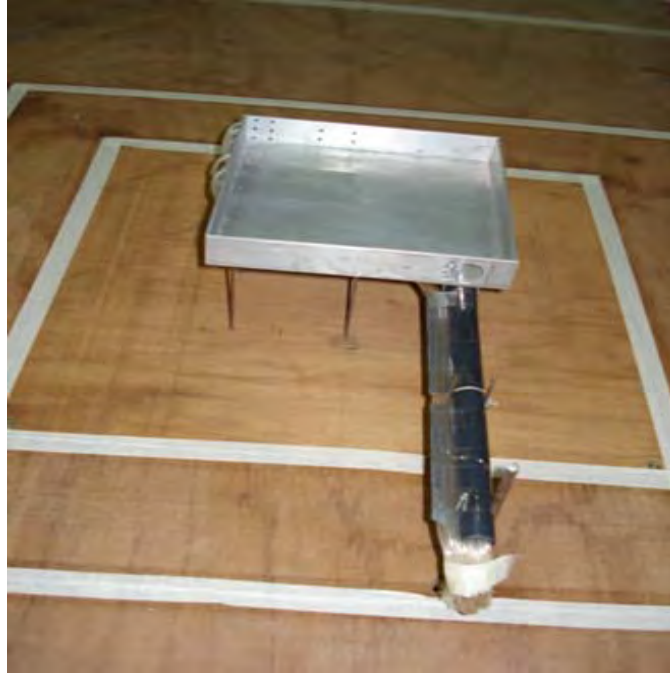
Figure 4.8: Distribution of pressure taps on the model with bundle of tubes and columns. (Photograph by the Author)
