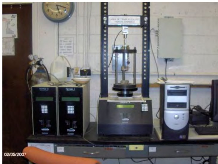
Figure 5.6 Equipment for unconfined compression test
