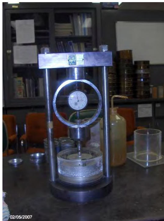
Figure 5.7 Soil volume change meter
