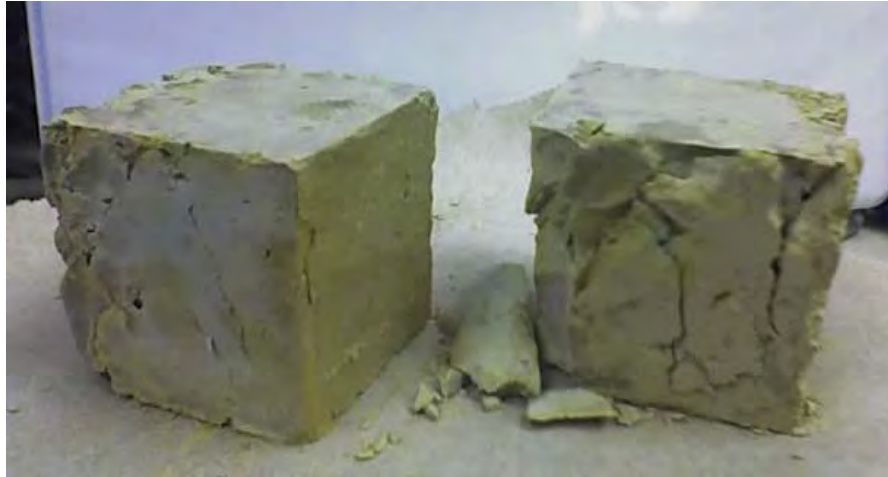
Figure 4.19 Failure modes of fly ash cubes during compression test
