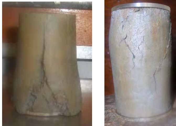
Figure 4.10 Failed samples of insitu base soil subjected to unconfined compression test.
