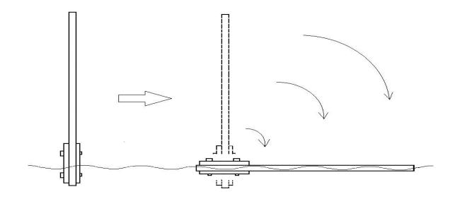
Figure 4: Repeated slamming apparatus and specimen
