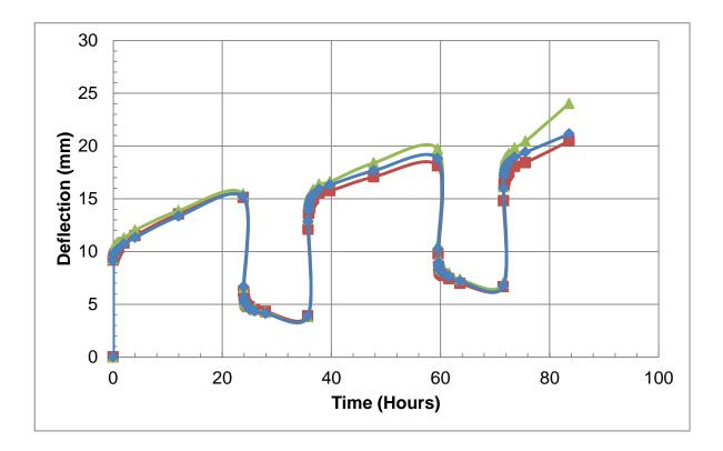
Figure 15: 24 hour loading and 12 hour unloading cyclic creep results
