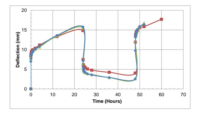
Figure 14: 24 hour loading and 24 hour unloading cyclic creep results
