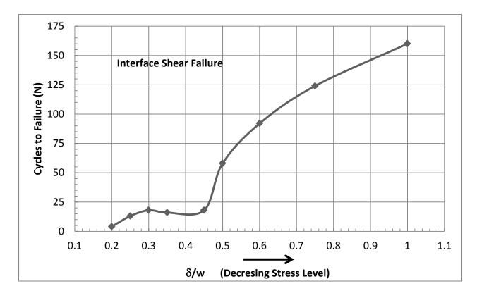
Figure 6: Average number of cycles to failure as a function of flaw size for *Type 1* specimens. No shift in modes of failure
