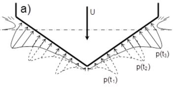
Figure 2: Wave slamming pressure distribution along V shape Wedge
