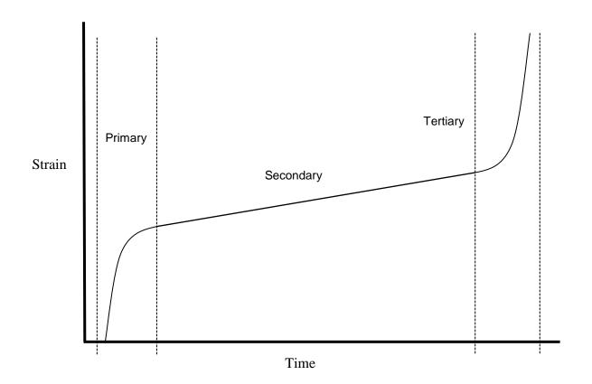
Figure 9: Typical creep phases
