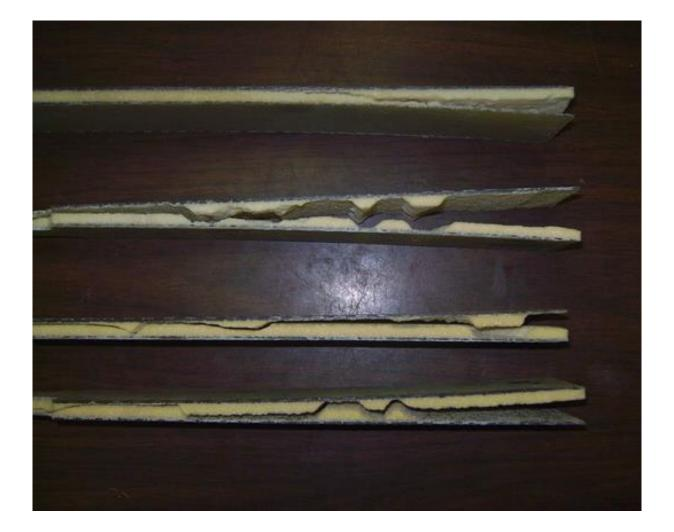
Figure 5: Typical interface and through the thickness shear failure in Type 1 Specimens
