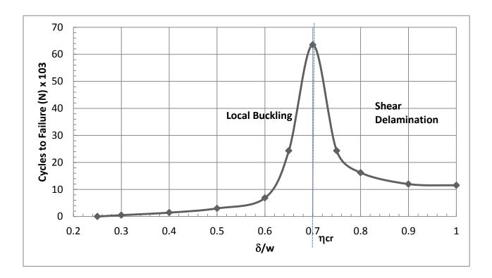
Figure 7: Average number of cycles to failure as a function of flaw size for *Type 2* specimens. Shift in mode and site of failure at the transition point  $\delta_{cr}/w$
