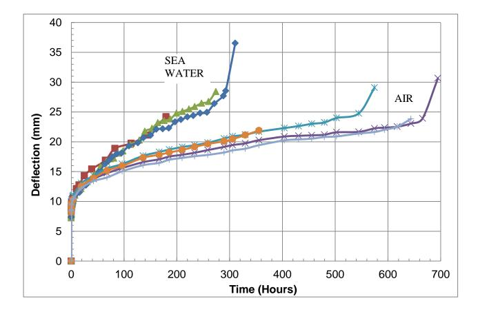
Figure 11: Comparison of Creep to failure in air and seawater
