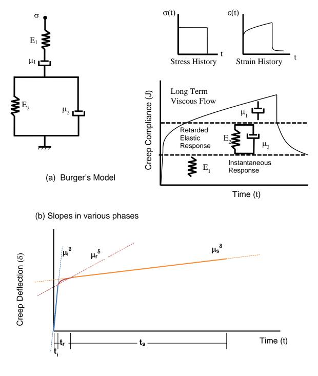
Figure 12: (a) Burger's model illustrating various stages of creep, (b)  $\delta$ -t curve and corresponding slopes.
