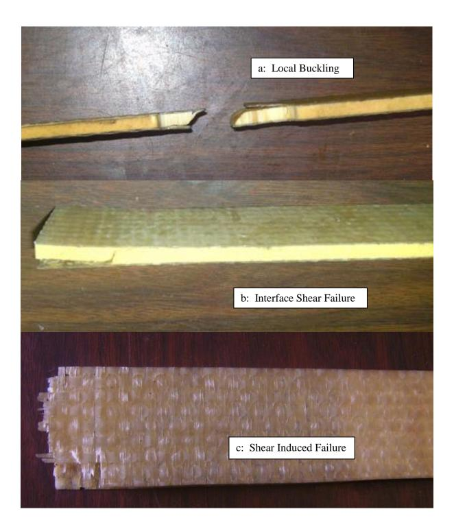
Figure 8: Typical (a) local buckling at the flaw site and (b,c) shear failure along the free end in *Type 2* Specimens
